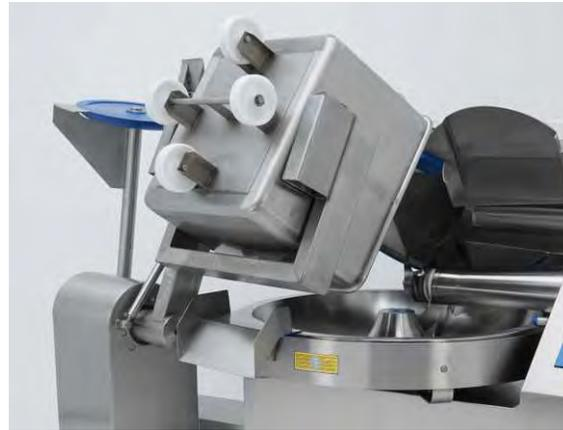
**Hydraulic loader** for fast and simple filling.
