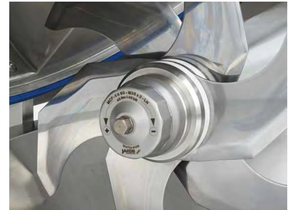
**Talsa Quicklock** reduces the time to dismantle and assemble the knives in the knife head.
